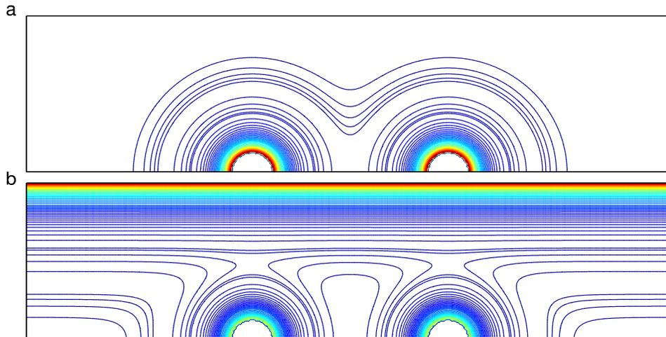
Figure 6: Two spheres confined in a charged cylindrical pore: calculated isopotential lines. A half-section of the physical geometry is shown, with the line of symmetry lying at the bottom. (a): Isolated spheres; (b): spheres confined in a pore. The pore wall is at the top.
