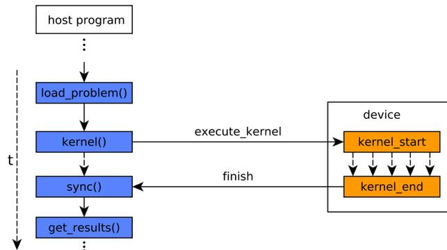
Figure 15: The GPU's main function, named *kernel*, is invoked from the CPU host code.
