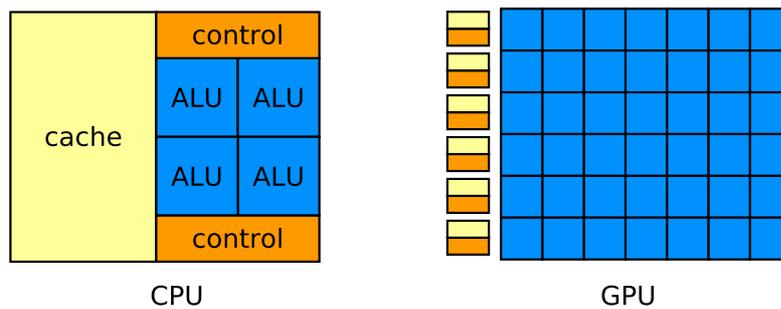
Figure 12: The GPU architecture differs from the one of the CPU because its layout is dedicated for placing many small cores, giving little space for control and cache units.
