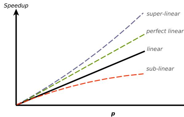
Figure 1: The four possible curves for speedup.
