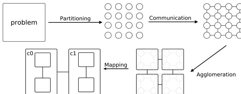
Figure 13: Foster's diagram of the design steps used in a parallelization process.
