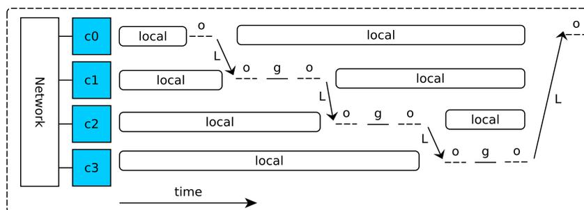
Figure 7: An example communication using the LogP model.
